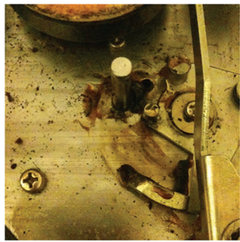
We removed old, often dry and hardened, grease and oil from Sony AV-3600/50 1/2" open reel decks and replaced them with synthetic grease and new oil.
