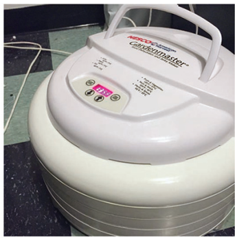
For tapes with sticky shed (hydrolysis) we clean then bake them in Nesco Gardenmaster Food Dehydrator. We seen the best results baking for ~40 hours at 135°F.
