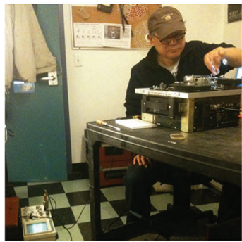
Gary Chang from GACC working on a Sony AV-3600 1/2" open reel deck. Here he's using an Hitachi Oscilloscope to measure the video outputs.
